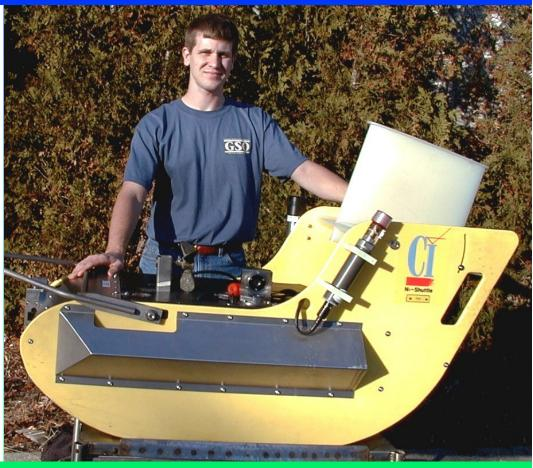
An undulating oceanographic recorder (above), towed behind a ship, is used to collect ecological parameters needed to assess the state of the marine ecosystem (left).
