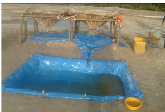
Photo 3 : Production system and bittern collection
